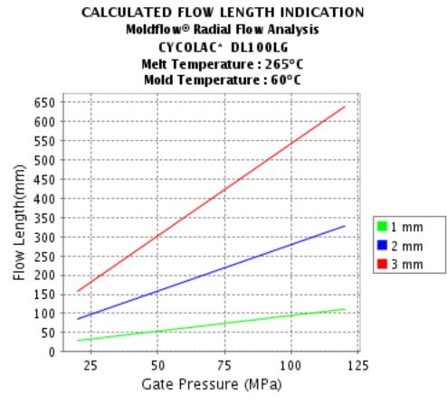
Note: Technical support is recommended if Gate Pressure is greater than 80 MPa. Contact your local representative. <sup>®</sup> Moldflow is a registered trademark of the Moldflow Corporation.
